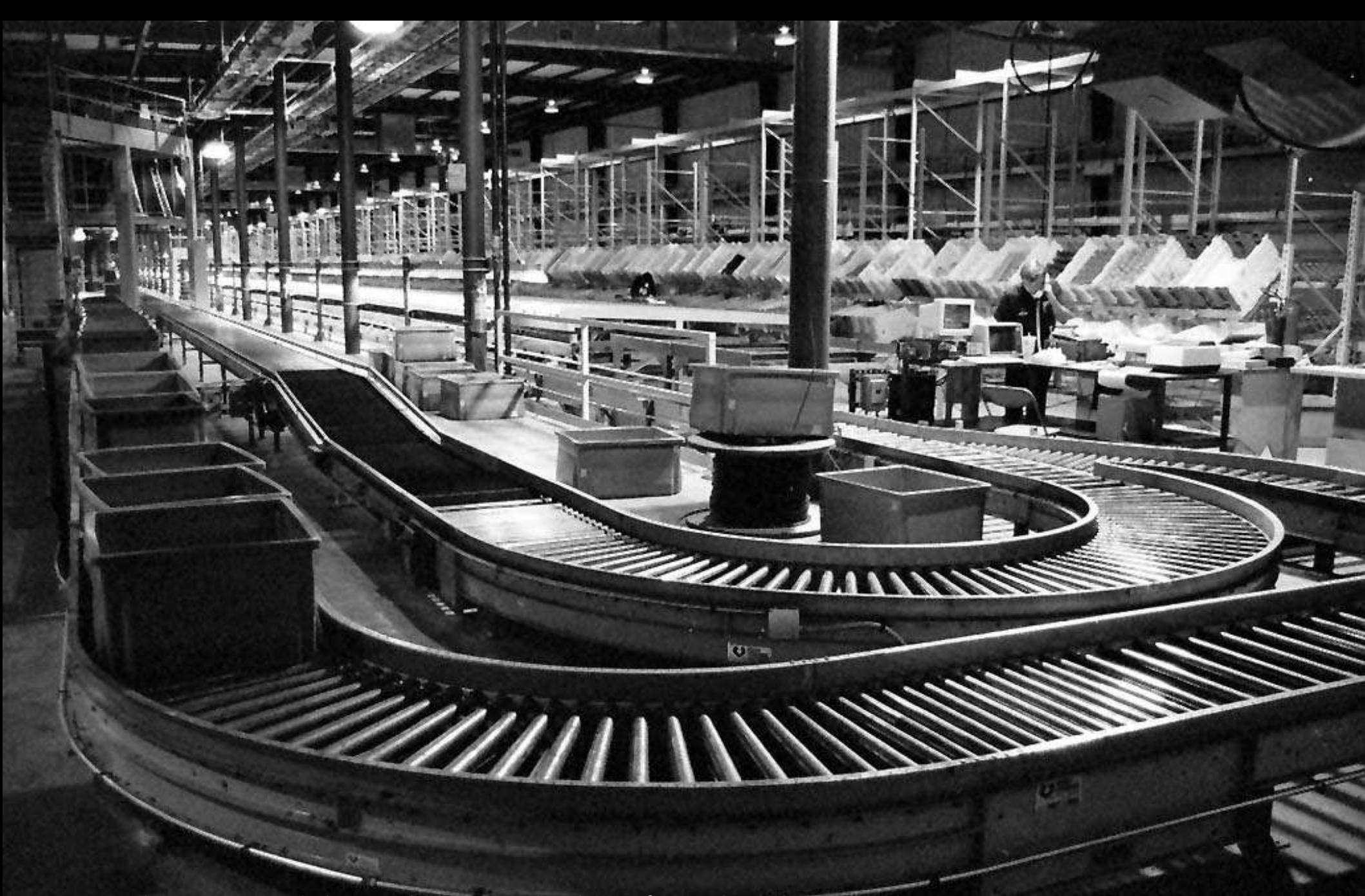
Around 1980 to 1990 I led team which invented and manufactured Robo-Pic high volume automated split case order filling system shown here at Tupperware plant in Halls, Tennessee
